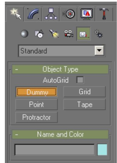
Now align the dummy to the centre of the wheel rim mesh by selecting the dummy and choosing the 'Align' icon. Now press 'H' to open the object selection dialog box and choose 'rim1' from the list.
